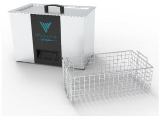
The Qi-400 is a 30Litre ultrasonic cleaner with a menu driven, LCD control panel. This allows simple adjustment of cycle time (0 to 99mins or infinity mode), temperature (ambient to 80°C), ultrasonic power and frequency mode
